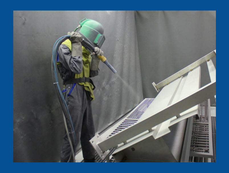
Sandblasting of surfaces is one of the most efficient ways of removing contaminants and preparing products for further treatment.
